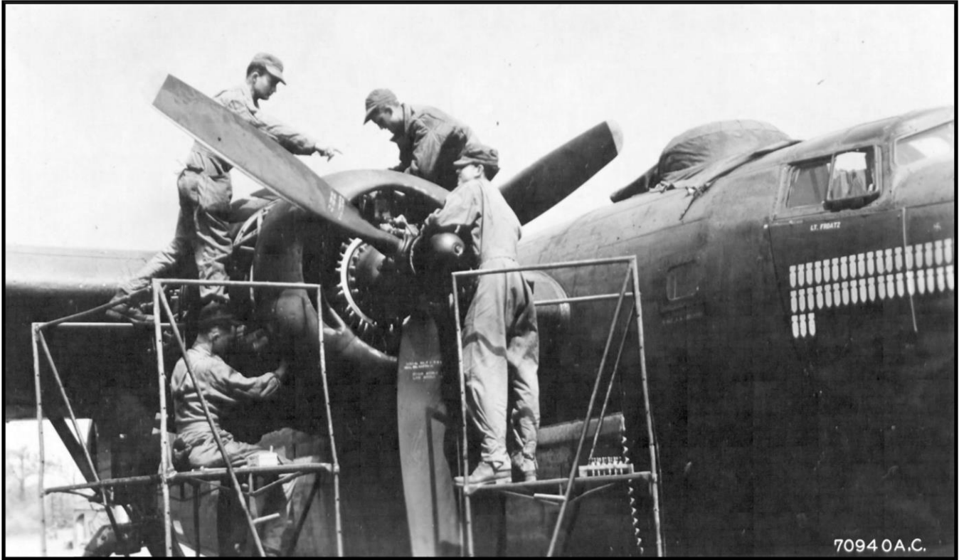
Maintenance crew of the 445 th Bomb Group work on the engine of a Consolidated B-24. Image courtesy of 445th Bomb Group Archives
