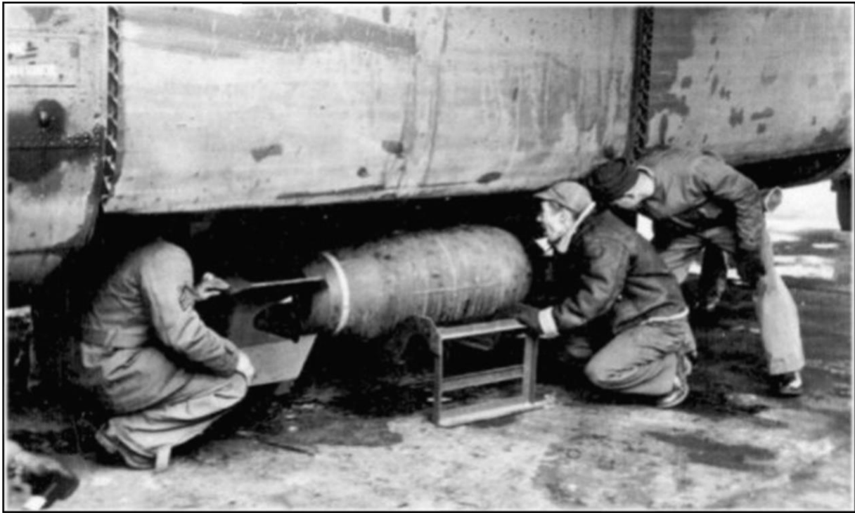
Ground Ordnance Crew loading B-24 with 2,000-pound general purpose bomb (2,000 lb. GP).
